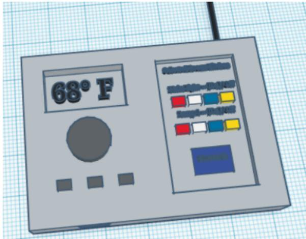
The second model was also created using TinkerCAD, and built on the preliminary with defined dimensions, curved edges, and a thinner design. The dimensions of this model were used to determine the final dimensions of the product.
