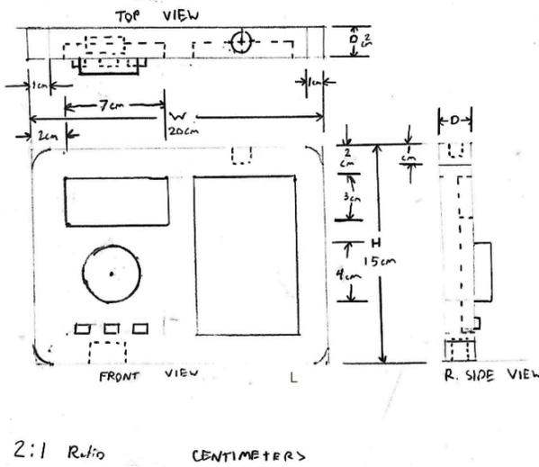
Figure 4: Dimensioned sketch of the device, based on the models above
